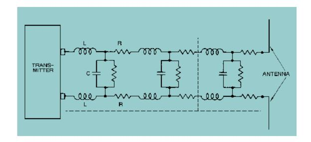
If the series inductance per unit length of line  $L_S$  and the parallel capacitance per unit length  $C_P$  are known, and the loss resistances can be neglected, one can calculate the characteristic impedance of a transmission line from the following equation:
